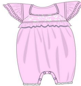
Fabrication 100% Cotton S/J 160 GSM Color Pantone 14-3209 TCX Size 9 Month -3 years Style Details ROMPER
