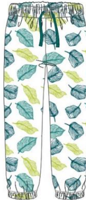
Fabrication 100% Cottonn S/J 160 GSM Size S, M, L, XL, XXL Style Details Pyjama
